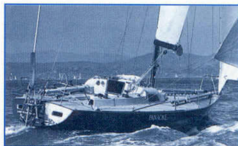
Panache, a 40-foot ultra-light Bill Lee custom design with a fin keel and spade rudder. As a winner of the Single-handed Transpac with the MONITOR as the only steering aid (no autopilots), the skipper reported successful windvane steering in surfing speeds up to 18 knots. The MONITOR steered the boat for 6-and-a-half days under spinnaker.
